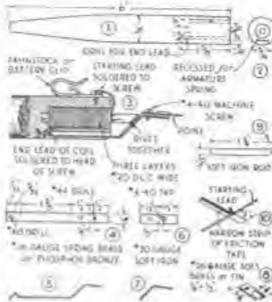
The handle, the assembled working point, and details of armature, spring, and other parts
